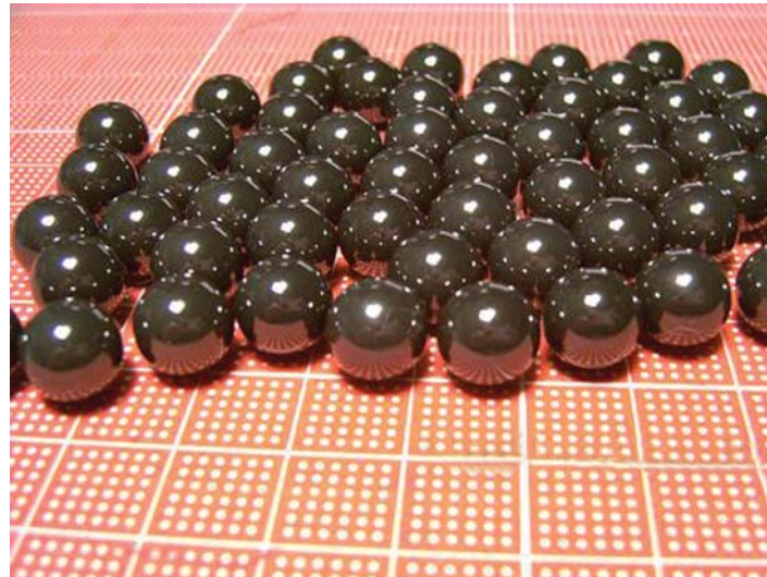
3.8-inch bearing balls used for fatigue test
